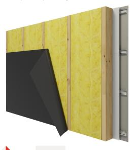
**2.** Slightly tighten the membrane and fix it to the structure using staples and nails with wide heads (tacks).
