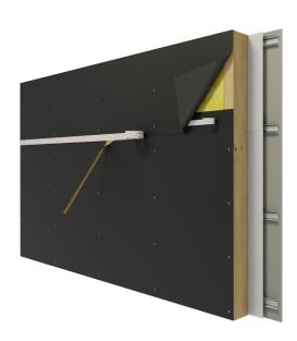
**5.** Provide a ventilation space of minimum width 2cm between the wind barrier and the façade.
